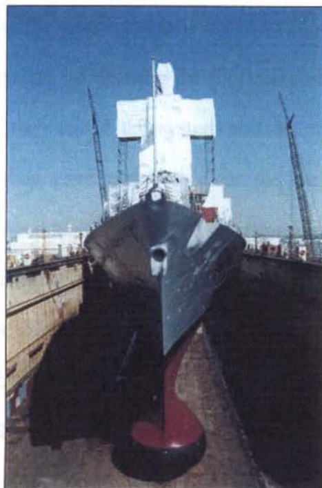
Figure 7. Sonar dome visible on a ship in dry dock. (From “Image,” 1998)
